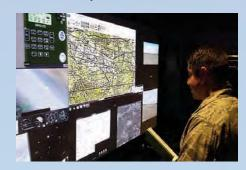
The system can be used independent of any running applications, and all the streams recorded during the action can be reviewed as needed. Instructors can use recorded missions to highlight and provide feedback, and "seek" to different bookmarks of the recorded action.
